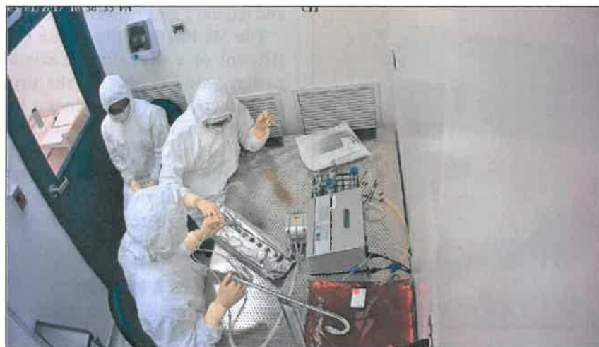
Figure 3. Custom aseptic filling and vial stoppering of a specialized product in Goodwin Biotechnology's ISO-5 cleanroom.
